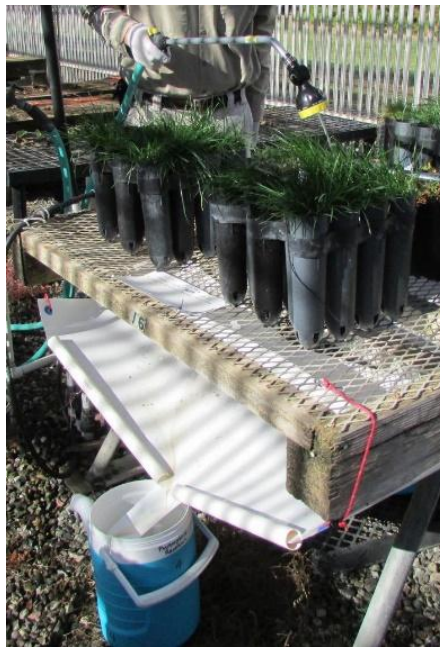
Figure 2: Irrigation using a calibrated watering wand. Plants are placed directly about the Runoff Collection Sheeting such that water drains into the Zoospore Collection Vessel. Photo credit: Phytosphere Research
