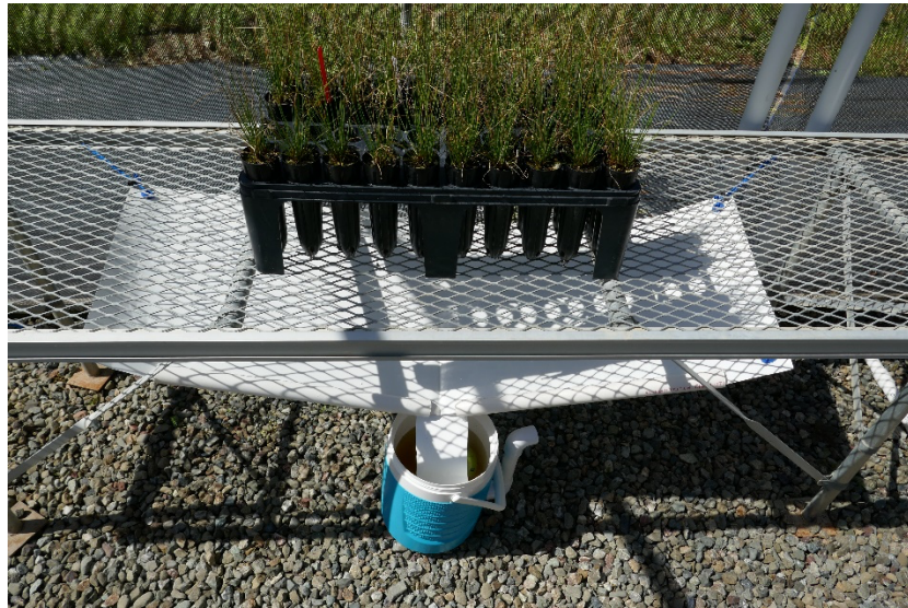
Figure 1: An in-progress leachate test, setup with a complete leachate collection system, single block of test plants, and a floating pear bait.
