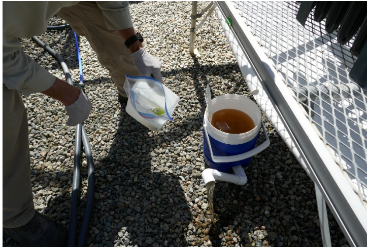
Figure 5: Collected leachate ready to be poured into a Ziplock bag and bucket for transportation and incubation.
