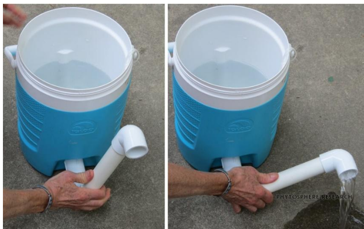
Figure 4. Proper drainage from the bottom of the Zoospore Collection Vessel. Photo credit: Phytosphere Research
